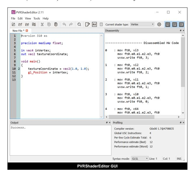
Shader disassembly for PowerVR Rogue graphics cores is provided within the tool. Developers can see the exact unified shader core (USC) instructions that have been generated by the compiler for the shader in question.
